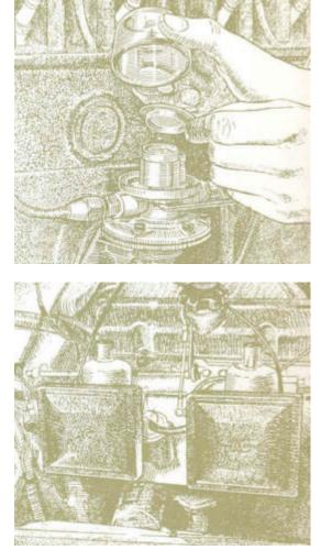
the air cleaner are fitted correctly in each case, since otherwise theses holes will be blocked
